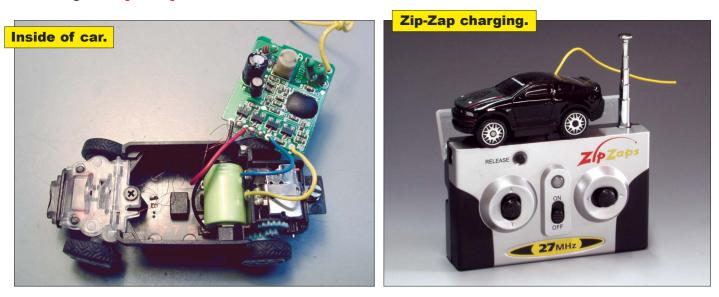
and Back buttons — that part can be carefully cut off if needed. The receiver, however, is pretty darned small at around 1" square and I'm sure that there may be many applications for this tiny four-channel device.
