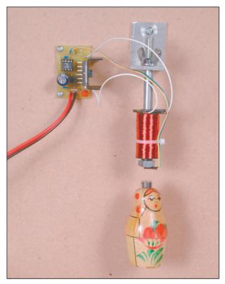
A FIGURINE OUTFITTED WITH A MAGNET dangles freely below an assembled version of Guy Marsden's magnetic levitation kit.
