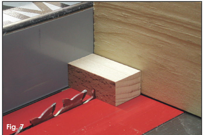
Cut out a section of the bearing support block on the table saw.
