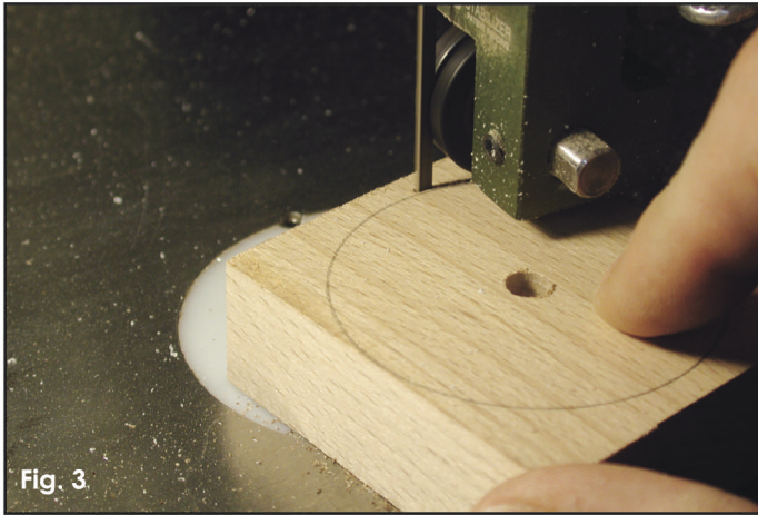
Cut out the circle on a bandsaw.
