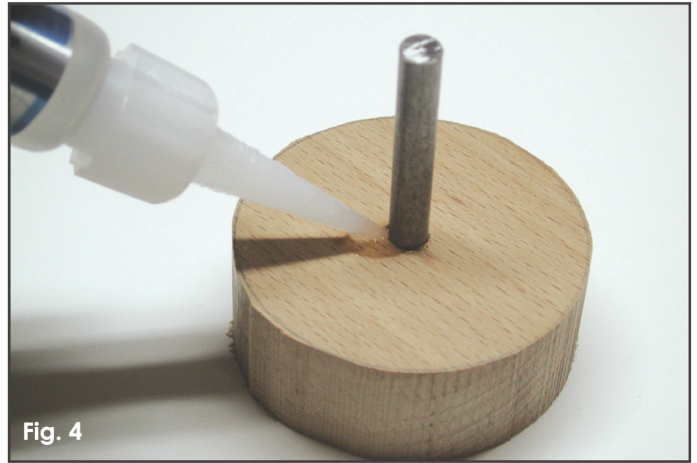
Glue the metal shaft in the hole with cyanoacrylate glue.
